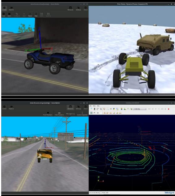
Figure 2: DDT's Virtual experimental Simulation (VxSIM), a physics-based modeling, simulation and analysis environment designed for advancing, training and testing AI and Autonomy systems. Supports sensor modeling, deformable terrain soil/regolith, parameter driven, multi-physics and ROS interface.
